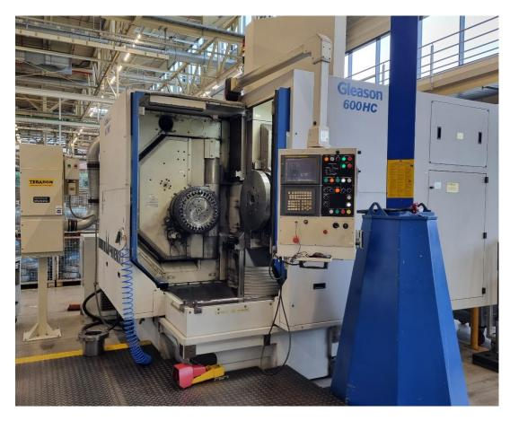
With the GLEASON PhoenixII® 600HC bevel gear cutting machine, manufacturers of medium-sized spiral and hypoid-toothed bevel gears can achieve faster cycle times and higher accuracies at lower workpiece costs.
